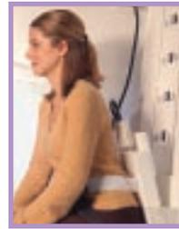
Quadrature Planar Coil with Lumbar Flexion Fixture (seated)
